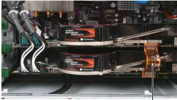
SLI bridge cable
